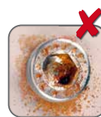
STAINLESS STEEL + NO STAINLESS STEEL= RUST
